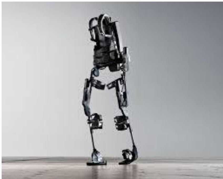
**Figure 1.** Design of the E-Helper exoskeleton.
